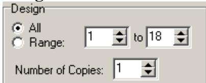
The design can be printed either in total or in part. To print only a part of the design change the range numbers.
